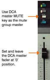
**ASSIGN channels or mix masters** to the DCA group using the DCA master **SEL** screen, channel **ROUTING** screens, or the DCA master **MIX** key ASSIGN function. If a channel is assigned to one or more DCA groups then its 'DCA' icon turns on.
